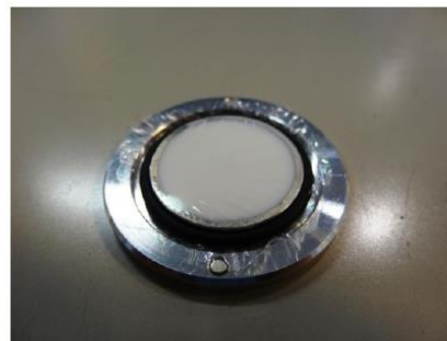
Fig. 1: Sunscreen lotion (left) and liquid sample holder filled with sunscreen lotion (right)
